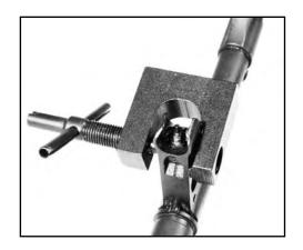
**Elevation Adjustments:** To move the point of impact up or down (elevation), position the slotted portion of the T-handle through the hole on the top of the sight housing and onto the sight post. Turn the T-handle clockwise to lower the sight post, counter clockwise to raise it. Raising the front sight will lower the point of impact. Lowering the front sight will raise the point of impact.
