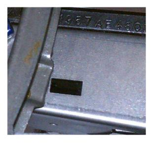
Use two 8-32 x 3/8 screws and nuts to secure the trunnion in the receiver to lock it in position before riveting. I would also recommend checking the fit of the recoil assembly in the trunnion to make sure the angle won't put it in a bind.
