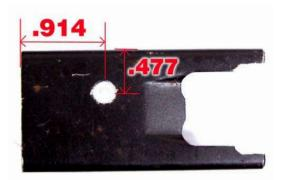
On trunnions with steps where the pin is drilled a clearance cut must be made. Machine the shelf so that you can drill the hole. You can check the level of the shelf by installing the trunnion in the receiver and look through the rectangle opening for the latch to see if it is even or slightly below the
