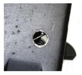
There is a notch in the pin that the spring locks into so the pin won't back out. The picture above shows the leg of the spring that will lock into the notch.
