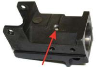
This was milled flat with a 7/32 end mill then drilled with #21 drill. Once the trunnion is riveted and all fitting has been done for the stock the trunnion needs to be "staked" to prevent the hinge pin from working out of the trunnion. Using a chisel or small punch displace the metal around the edge of the pin enough to keep it from coming out.
