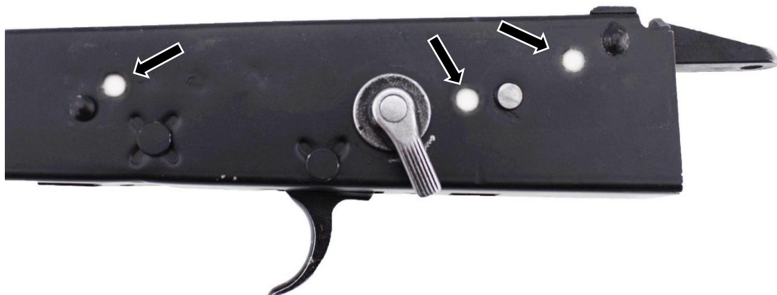
Figure: 11 hole placement after drilling with the 13/64 inch drill.
