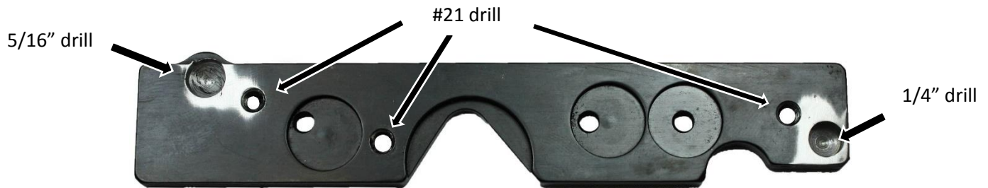
Figure: 8 counter drill holes for rivet heads and drill thru anchor plate at datum "C" (2x) & "D"
