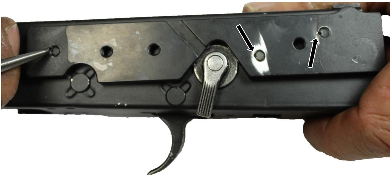
Figure: 15 “ping” a divot into the screw threads to keep from backing out.
