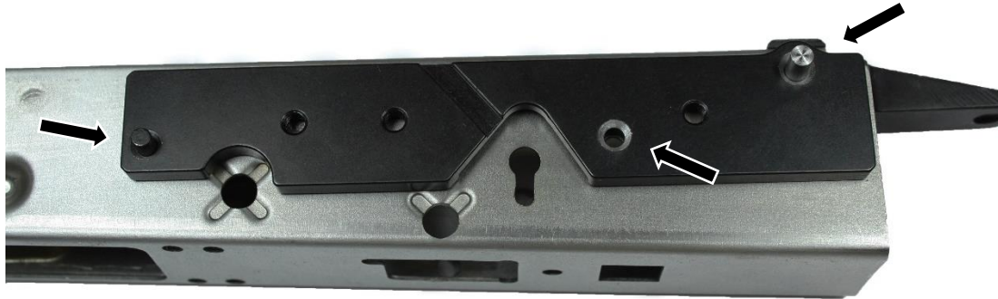
Figure : 3 drilled and countersunk datums “A”, “B”, “D” Drilled datum “D” thru receiver
