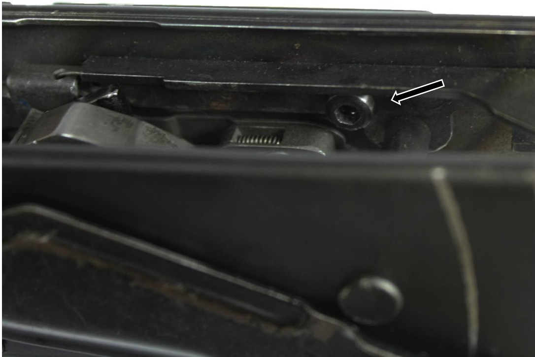
Figure: 13 Longer screw head ground down to clear hammer
