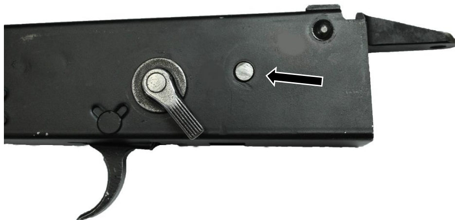
figure: 2 ground trunnion rivet for clearance
