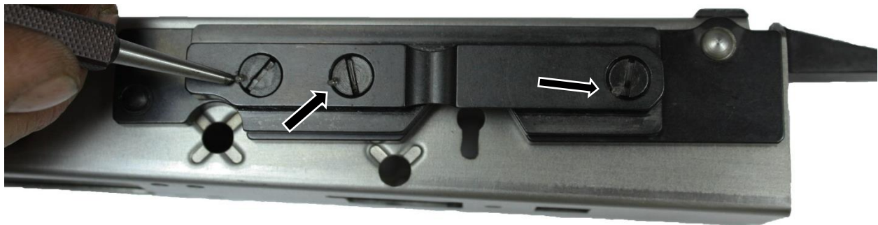
Figure : 6 center punched screw heads
