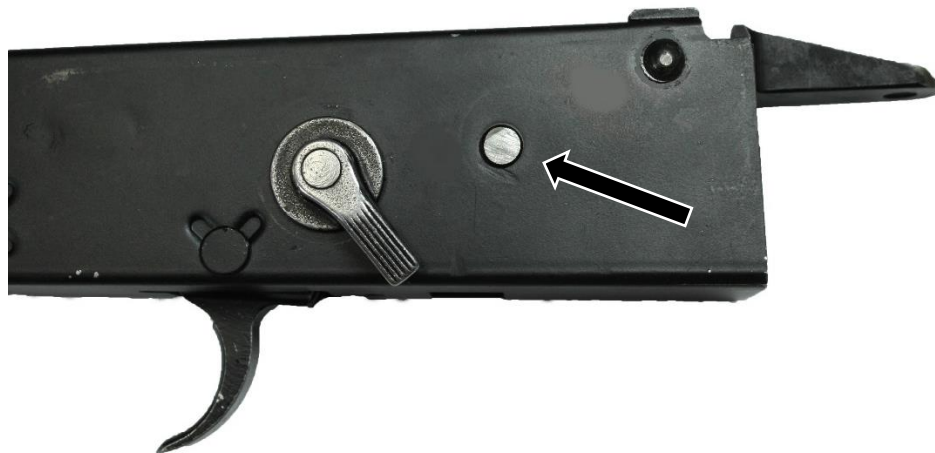
figure : 9 ground trunnion rivet for clearance
