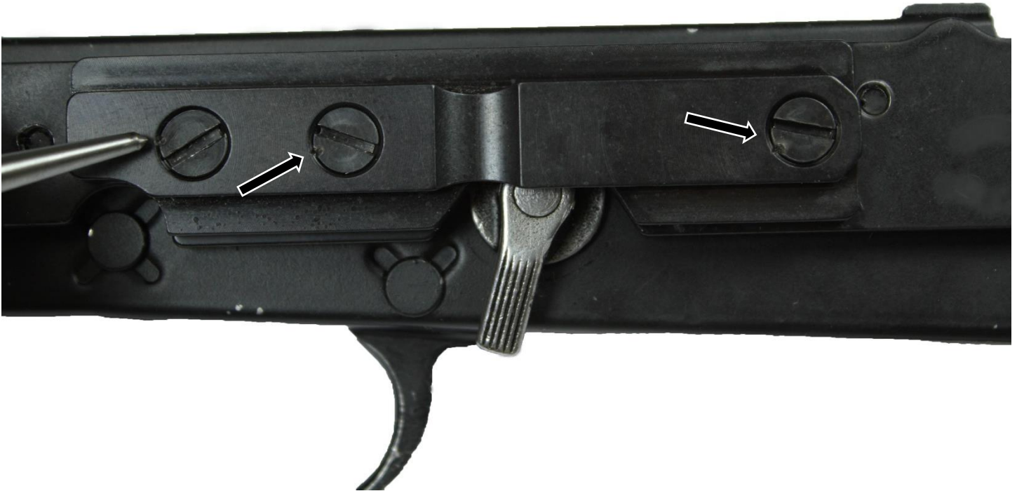
Figure : 16 center punched screw heads to keep from backing out
